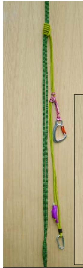
← **Figure 2A.** A rated, short webbing sling (red) is girth-hitched to a rated, fixed-eye carabiner (“rated” means that the ratings for that piece of gear meet the requirements of ANSI Z133.1-2006.) The short webbing sling is then attached to the primary tether with a three-wrap, six-coil Prusik knot. The webbing sling provides an adjustable attachment point on the tether.
