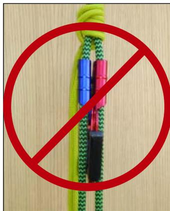
**Figure 10B.** A system that should not be used! The ascenders create a spread in the doubled line, and the friction hitch has to be very, very loose. If something prevents either one of the cams from holding on the line, the climber will most likely continue to hold the ascender and will fall to the ground.
