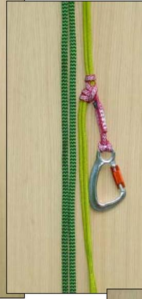
loop serves as a stopper knot for the webbing. The key chain carabiner at the bottom of the tether can be clipped to the saddle to prevent the end of the sling from becoming entangled in the climber’s feet while
