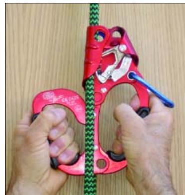
**Figure 6. The cams of the Kong Twin can be prevented from opening by placing a key chain carabiner (blue) in the small hole behind the cams.**
