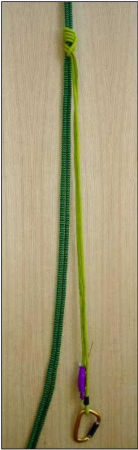
**Figure 1.** A Prusik loop consists of a length of cord formed into a loop by tying the ends together with a grapevine knot. The loop is attached to the doubled climbing line with a friction hitch (here a three-wrap, six-coil Klemheist).
