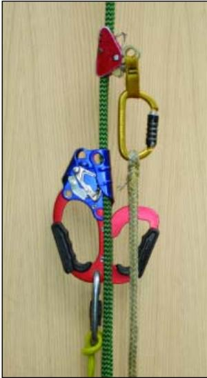
**Figure 9.** Another method to back up the Kong Twin is to place a Dualcender above the Kongs and use a separate tether to attach the climber to the Dualcender. This creates a backup system (the Dualcender) that is completely independent of the primary (the Kongs).
