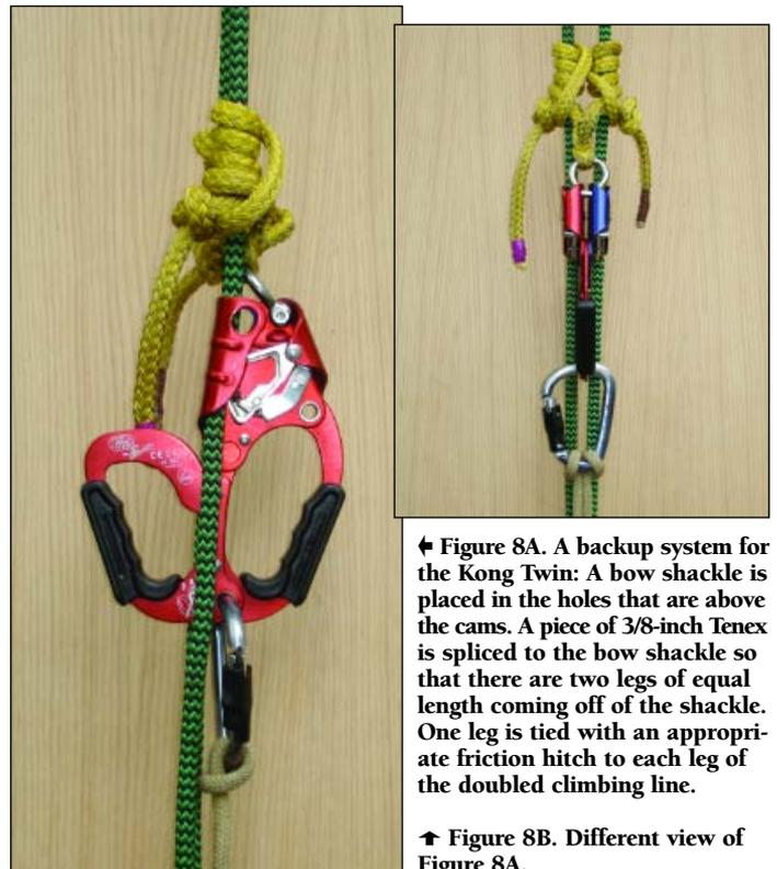
◀ **Figure 8A. A backup system for the Kong Twin: A bow shackle is placed in the holes that are above the cams. A piece of 3/8-inch Tenex is spliced to the bow shackle so that there are two legs of equal length coming off of the shackle. One leg is tied with an appropriate friction hitch to each leg of the doubled climbing line.**
