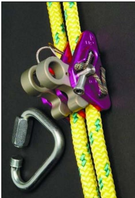
**Figure 4. The Footlocker is an ascender that has a quick-release pin and twin cams for use on a doubled line. The drawback is that the cams are locked together with either a carabiner or a delta link (pictured). When one cam moves, the other cam also moves. If the climber pulls down on either leg of the doubled line, both cams open and the entire unit—along with the climber—falls to the ground.**
