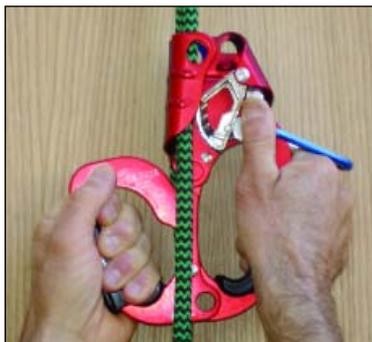
**Figure 7. Even with a key chain carabiner behind the cams, the climber can accidentally release the cam with his or her thumb (as pictured), or debris of some sort can prevent the cam from properly and completely engaging on the rope.**
