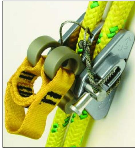
**Figure 5. The Dualcender also has two side-by-side cams, but there is a single piece of webbing connected to both of the cams. The climber's carabiner is attached to the bottom of the webbing. This allows the climber's weight to "float" between both cams. If either leg of the rope is pulled, the one cam that is on that leg of rope will be released, but the other cam will remain engaged.**
